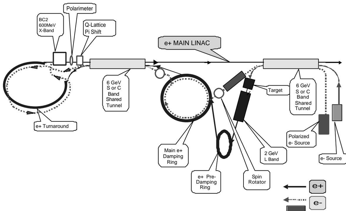
Figure 14.4: The direction reversal model. From [14].
