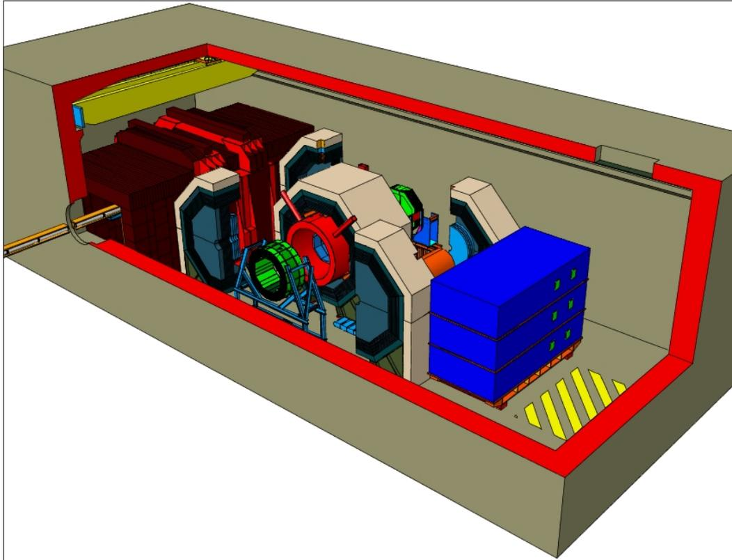
Fig. 5.2: Picture of the experimental hall during the assembly of the detector. (The beam line is shielded with concrete blocks. One half-barrel calorimeter and one end cap calorimeter and the TPC are in preparation on maintenance supports.)
