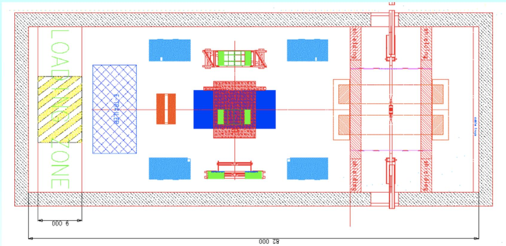
hall and are stored in the 9m by 30m loading and storage zone (see Fig. 3.1 and Fig. 3.2). Two cranes with a capacity of 80t each are foreseen for the handling of heavy items in the experimental hall. Fig. 9.4 (Appendix) shows a sketch a possible civil engineering solution for the underground hall construction.
