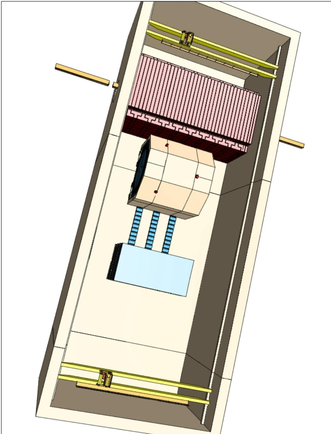
Fig. 5.3: Closed detector in the park position.
