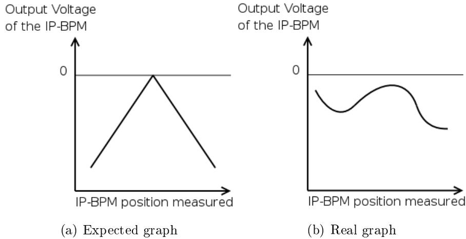
Figure 2: Response of the cavity versus offset
