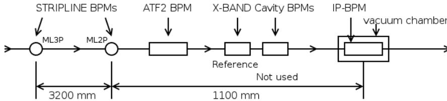
Figure 1: The setup of the LINAC end
