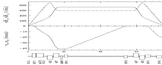
Figure 1. Optics of the extraction line.
